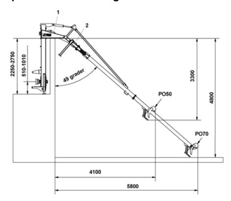
The sketch is indicated with the maximum extent of the top brace and the tower perpendicular to the slurry pit.
